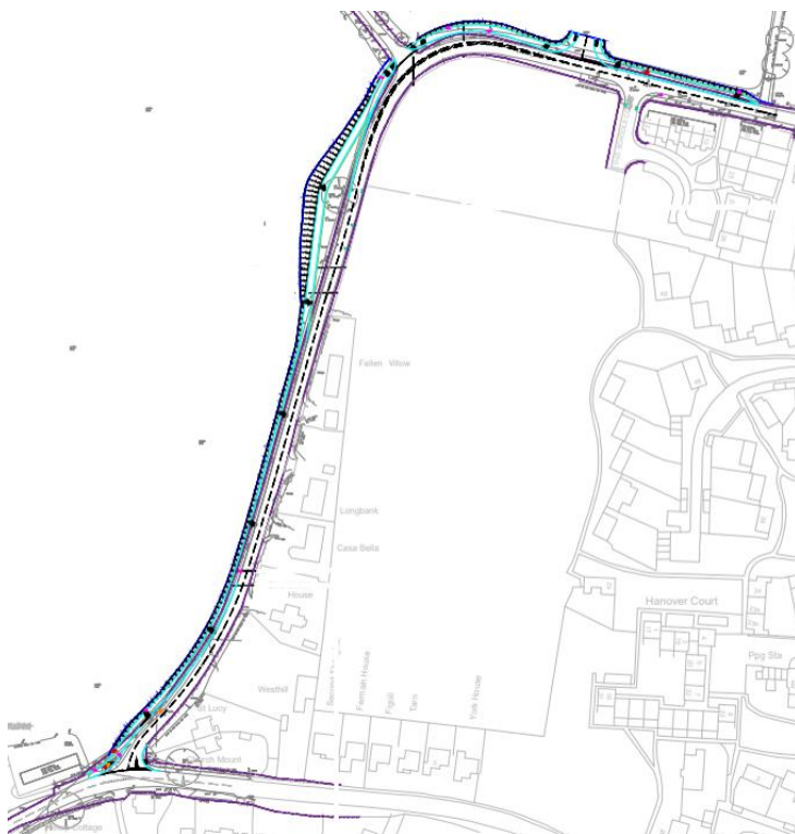
Figure 3.4: Planned Footway/Cycleway Improvements on School Road
