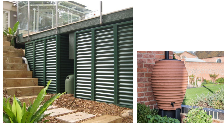
Figure 41: Examples of concealed tanks used for rainwater harvesting
