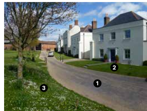
Examples of edge lanes in Dorchester, with low-speed roads shared between motor vehicles and cyclists, and opportunities for on-street parking (note: some localities may prefer clearly defined footways and parking bays).
