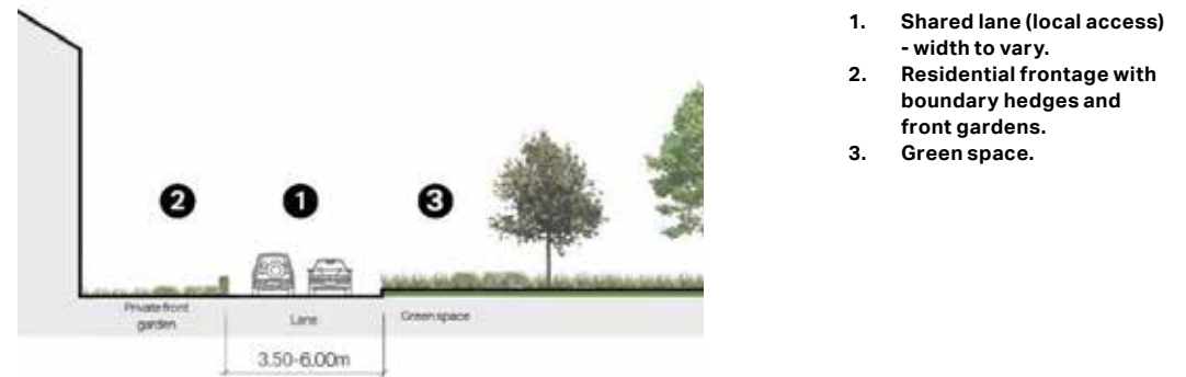
Section showing indicative dimensions for edge lanes. The lane width may vary to discourage speeding or provide space for parking.
