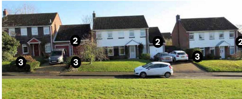
Figure 43: Example of on-plot garages along Marsh Road. The height of the garages is no higher than the main roofline of the buildings, whilst planting and vegetation in the front gardens help improve the visual result and give the impression of a less car dominated place.
