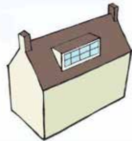
Loft conversion incorporating a long shed dormer which is out of scale with the original building.
