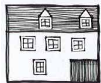
Loft conversion incorporating gabled dormers which are out of scale and do not consider existing window rhythm nor frequency.
