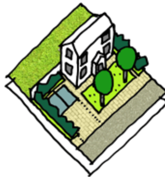
On-plot parking on driveway
