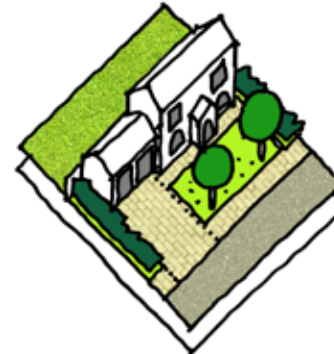
On-plot parking in garage
