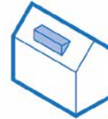
Loft conversion incorporating a long shed dormer which is out of scale with the original building.
