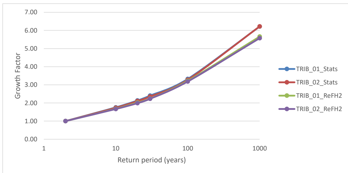
Figure 5-1 Comparison of growth curves between the FEH Statistical and ReFH2 methods
