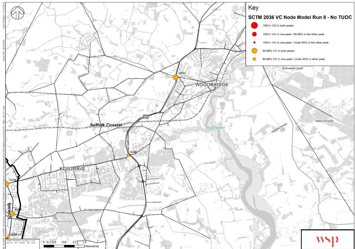
Figure 9 - Martlesham & Woodbridge – MR8 without TUOC, Junctions with Overall V/C over or near capacity
