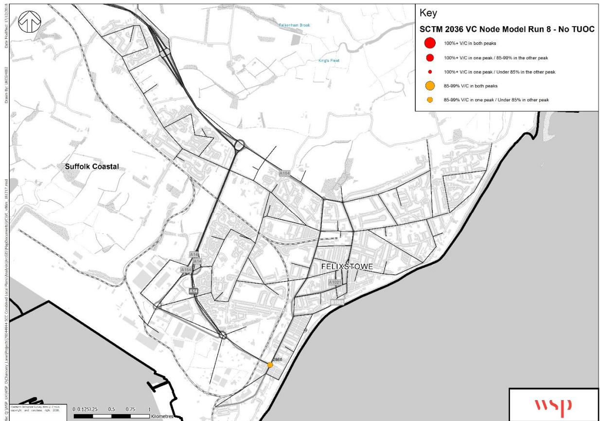
Figure 6 - Felixstowe – MR8 without TUOC, Junctions with Overall V/C over or near capacity
