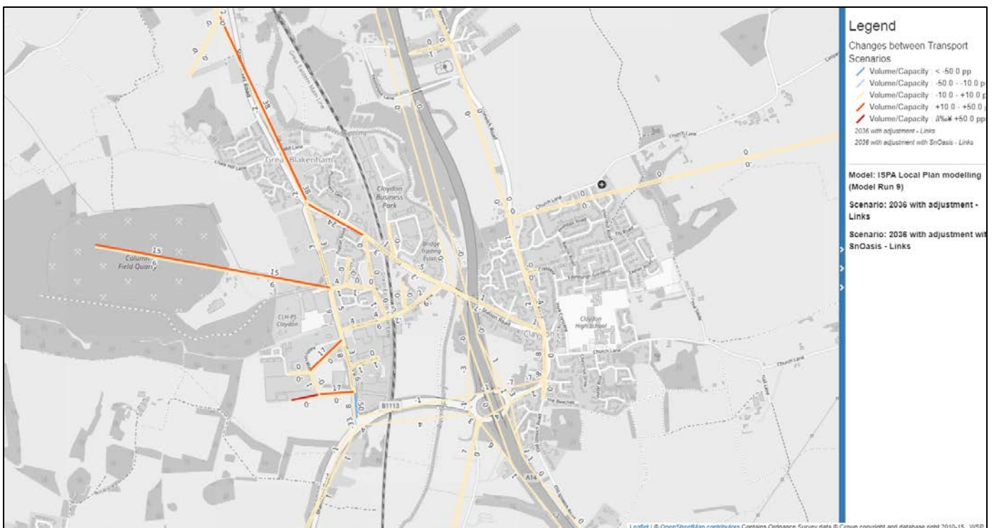
Figure 11: 2036 Local Plan Scenario, With SnOasis vs Without SnOasis, V/C Difference, PM Peak
