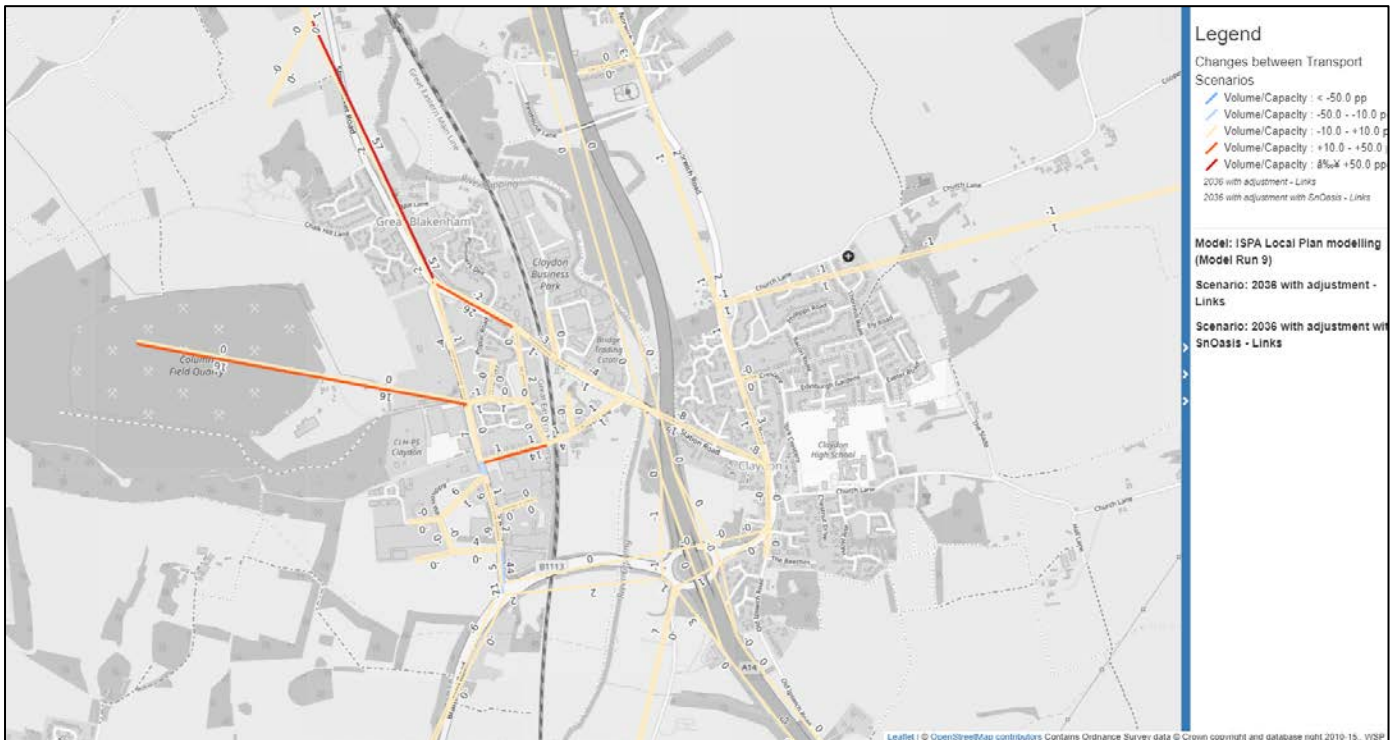
Figure 9: 2036 Local Plan Scenario, With SnOasis vs Without SnOasis, V/C Difference, AM Peak
