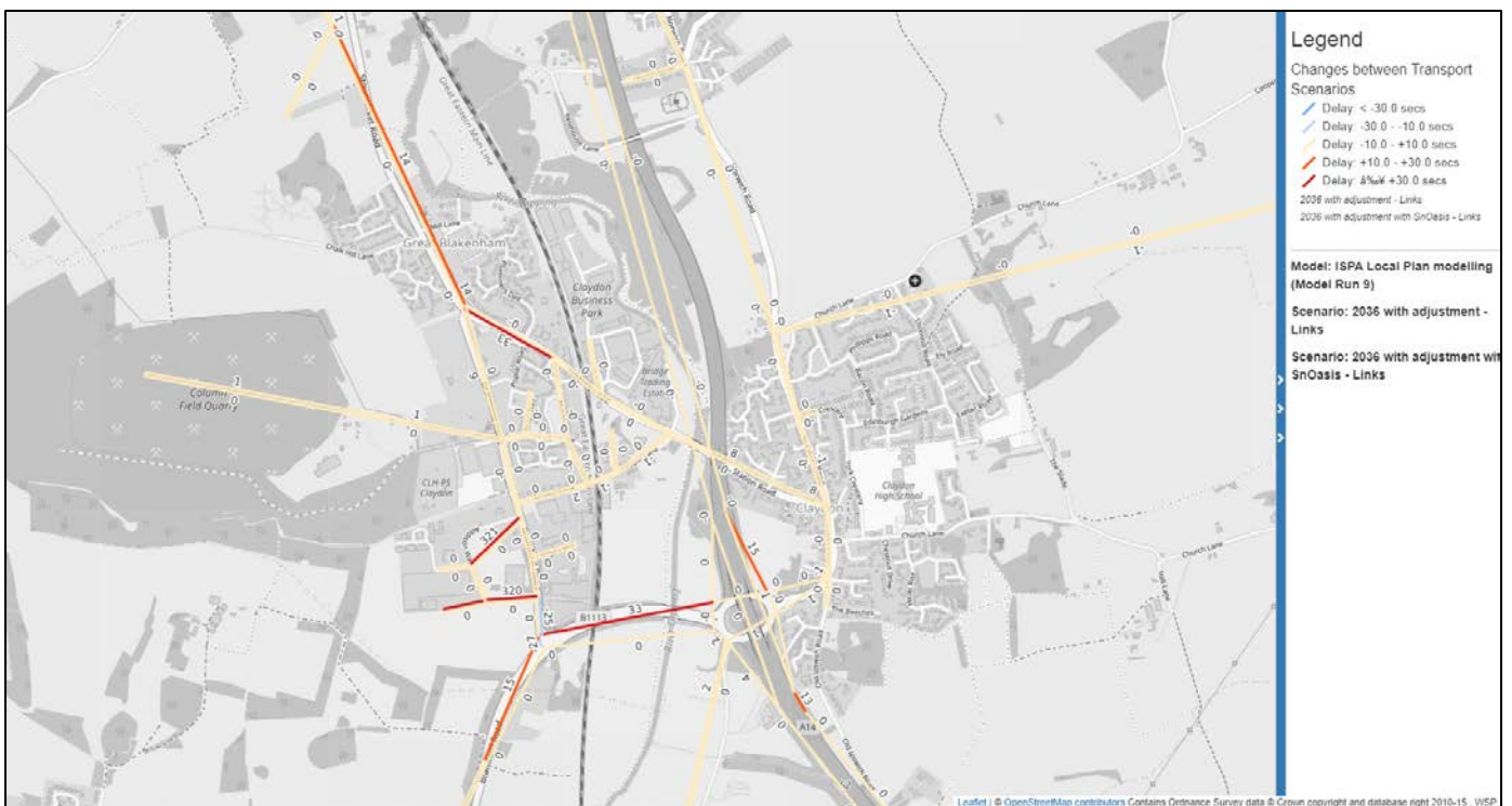
Figure 8: 2036 Local Plan Scenario, With SnOasis vs Without SnOasis, Delay Difference, PM Peak
