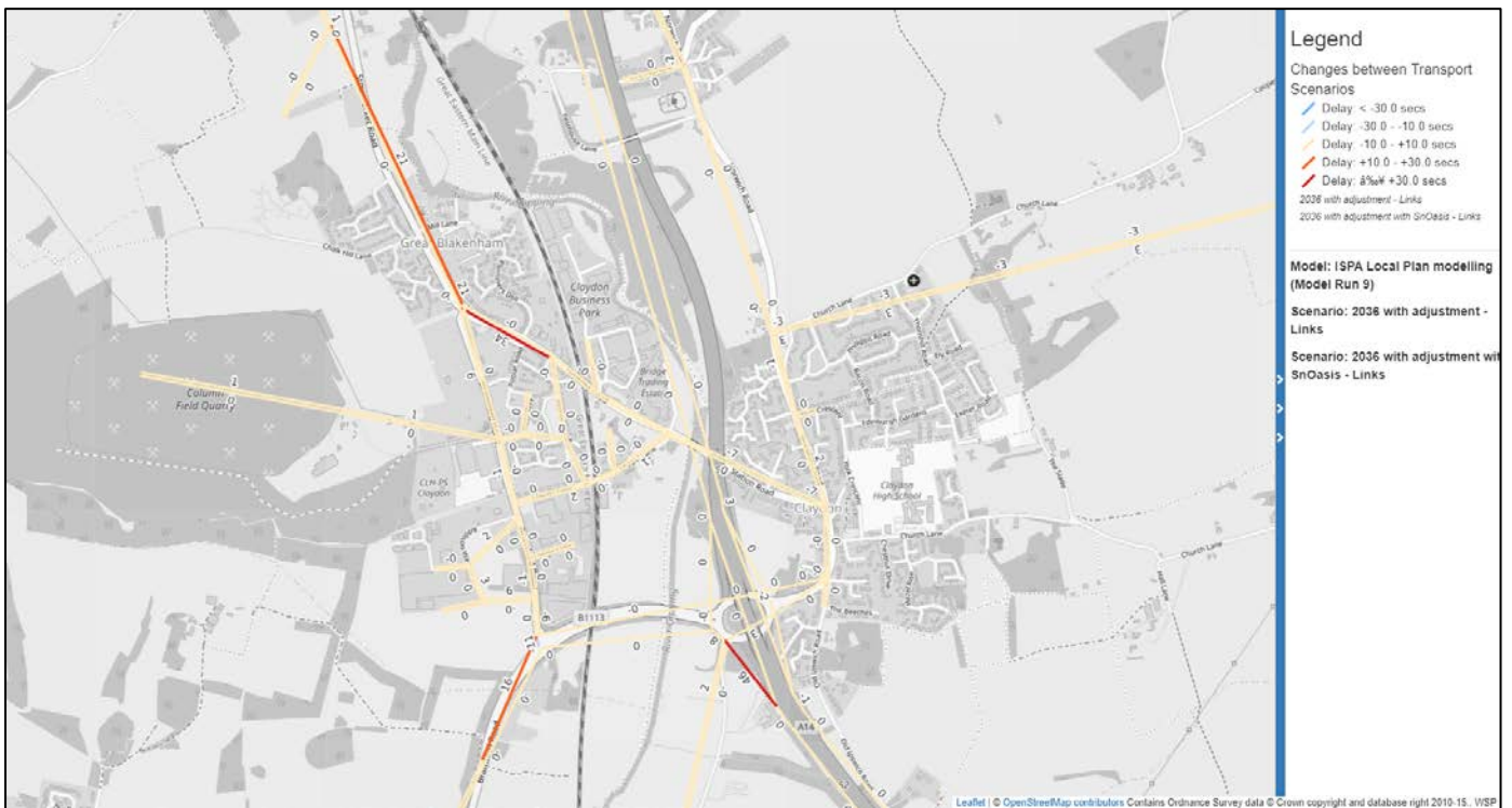
Figure 7: 2036 Local Plan Scenario, With SnOasis vs Without SnOasis, Delay Difference, AM Peak
